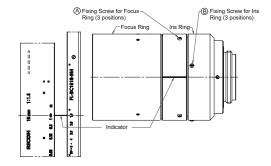
For setting the focus correctly, the CalibrationGrid should be placed in the middle of the working range. Then, the focus ring should be turned until the bars in the images become a minimum. After focusing in this way, the grid should be placed at the minimum and maximum working distance.
